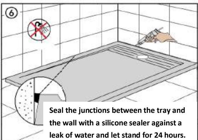
Seal the junctions between the tray and the wall with a silicone sealer against a leak of water and let stand for 24 hours.
