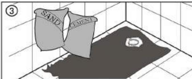
Ensure the base of the tray is completely solid and level with unpolished terrazzo or second-rate mortar.
