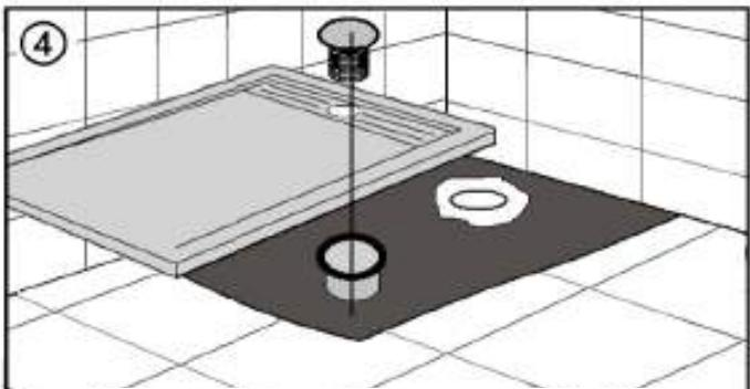
Protect the walls with adhesive tape to not stain and install the valve.
